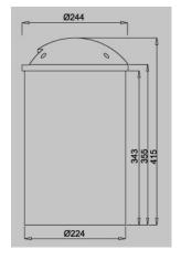
The N08 Ground embedded light is an attractive inground light featuring a die-cast aluminium construction for directional lighting effects. It also comes equipped with a specialised reflector system and shock resistant toughened glass cover.
